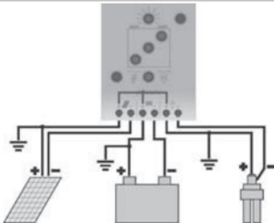
Be aware that the positive terminals of the CML controller are connected internally and therefore have the same electrical potential. If any grounding is required, always do this on the positive wires.
