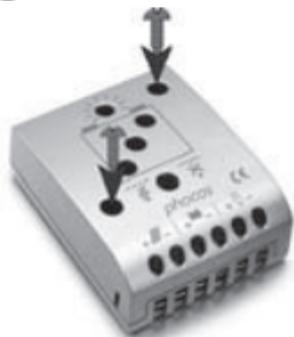
Mount the controller to the wall with screws that fit to the wall material. Use screws with 4 mm shaft and max. 8 mm head diameter, no counter sink. Mind that the screws have to carry also the force applied by the wiring.
