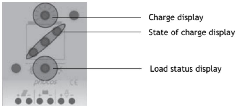
In normal operation, the controller shows the state of charge of the battery and the charge from the solar panels. Any change of the state of charge (SOC) to a lower status is additionally signaled acoustically.
