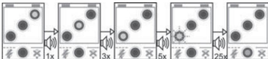
The loads are disconnected approx. 1 minute after a series of 25 signals.
