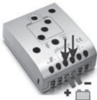
Connect the wires leading to the battery with correct polarity. To avoid any voltage on the wires, first connect the controller, then the battery. Mind the recommended wire length (min 30 cm to max approx. 100 cm) and the wire size:
