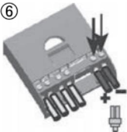
To avoid voltage at the load terminal, push the button to shut off the load output. Connect the wires leading to the loads with correct polarity. Mind the recommended wire size:
