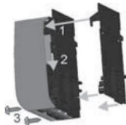
Mount the controller to the wall with screws that fit to the wall material. Use screws with 4 to 5 mm shaft and max. 9 mm head diameter, no counter sink. Mind that the screws have to carry also the force applied by the wiring. Mind also the minimum required distance to floor and ceiling, this is necessary for ventilation reasons.
