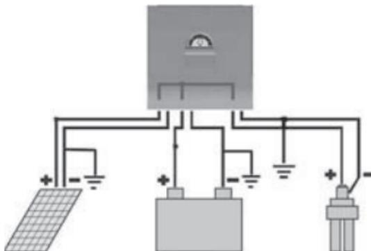
Be aware that the CXN is negative grounding and the negative terminals of the CXN controller are connected internally and therefore have the same electrical potential. If any grounding is required, always do this on the negative wires.
