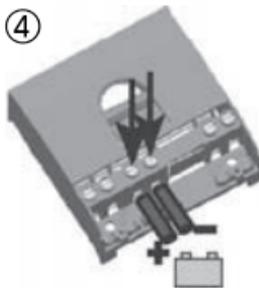
Connect the wires leading to the battery with correct polarity. To avoid any voltage on the wires, first connect the controller, then the battery.
