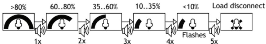
The percentage corresponds to the available energy until Low Voltage Disconnect in relation to a fully charged battery.
