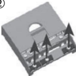
Remove the screws from the strain relief and take off the strain relief bridges.
